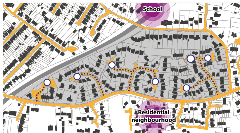
Figure 3.3.3 Creating cul de sacs creates longer journeys to school and encourages driving
